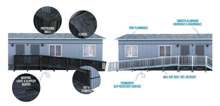
Another point of strife regarding wood ramps is their potential to fall out of alignment with the ADA's guideline concerning a maximum slope of 1:12. Due to warping and shifting boards, the slope of a wood ramp could become very inconsistent and potentially exceed 1:12. Conversely, aluminum ramps can be set at a continuous 4.8 degree angle, allowing the ramp to maintain the 1:12 slope throughout its lifecycle. [source]
