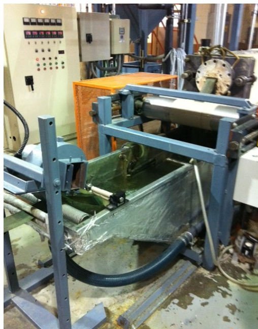
View of extruded sheet entering "quench bath" to cool and solidify the plastic
