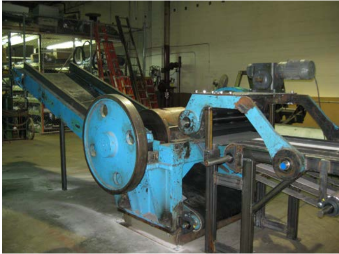
AstroTurf Turf Chopping Machine, Dalton, Georgia. This is an example of the machinery used to “chop” the field into smaller pieces so the material can be reprocessed. Currently, AstroTurf uses a local, outside firm to do this initial processing of its internal turf waste and fields brought in for recycling
