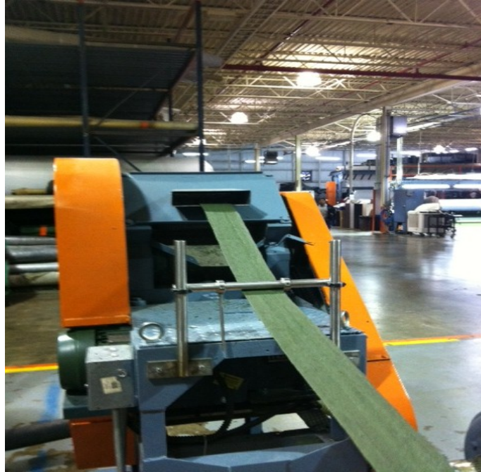
View of sheet entering final “chopping” process, which allows for re-pelletizing. The new pellets can be extruded into products or ground and used as granules.
