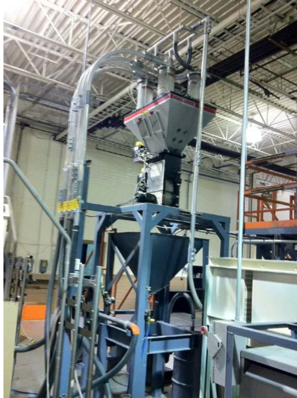
View of the second extruder, which combines virgin PE and MasterBatch.
