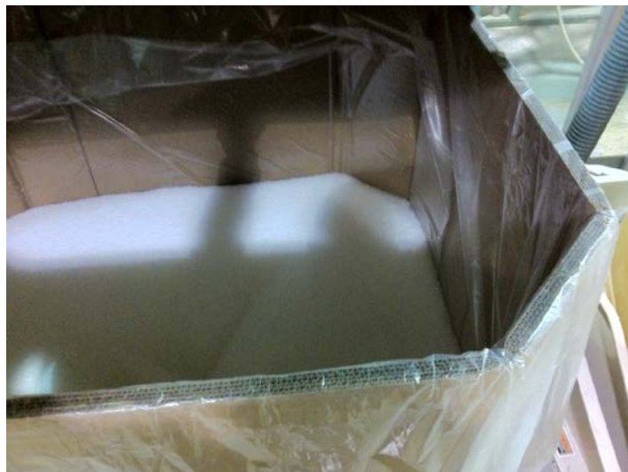
View of virgin PE pellets being sent into the second extruder. These will be mixed with Master Batch.
