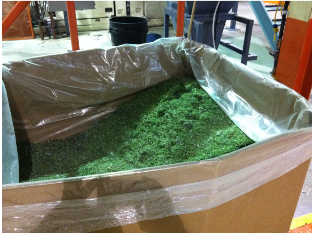
Final form the field takes prior to recycling extrusion process. The process allows only for approximately 5% of the infill to remain in the turf.
