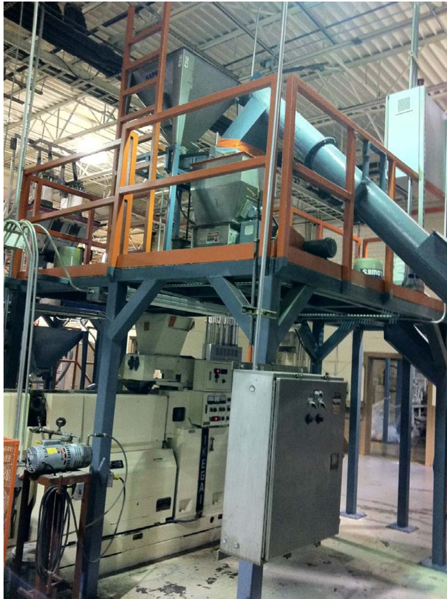
View of the extruder melting the turf "chop" at UTT Dalton, GA 2012 Note: The second extruder can be seen in the top left-hand side of the photo. Both extruders feed into the center screw that can be seen behind the control panel at the bottom of the photo.
