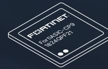
As a co-processor to the main CPU, Content Processors offload resource-intensive processing and drive content inspection to accelerate security functions.
