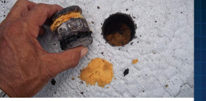
**Core Cut Analysis** – We are able to provide non-destructive core cuts. Core samples involve cutting through the membrane of the roof down to the deck. These samples can provide information on the existing roof assembly, including type of roof, type of insulation, amount of insulation, and type of substrate.
