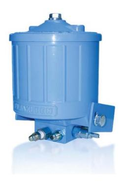
Filtakleen Bypass Hydraulic Oil Filters permanently maintain hydraulic oil at ISO 14/11 H20=<0.05%. The Filtakleen system can be either installed directly onto the machine or used as an off-line cleaning rig to purify the oil. The benefits to the oil and machine are two-fold: Ultra-fine Debris removal down to 1 micron which, is generally missed by the primary 10-micron filter.
