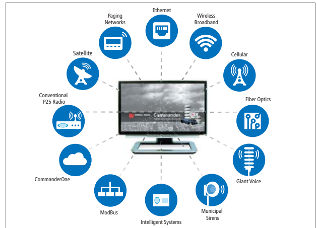
Commander® On-Premise Siren Control and Messaging System (SFCD)
