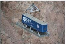
**Transformer Oil Processing Units** – To operate reliably and safely, transformer insulating oils must be maintained to preserve their original operating characteristics. In addition to Shermco's extensive laboratory services, we have several transformer oil processing trailers that can be dispatched to your location to filter, dehydrate and de-gas your oil, often avoiding costly replacement and extending the service life of your transformers.
