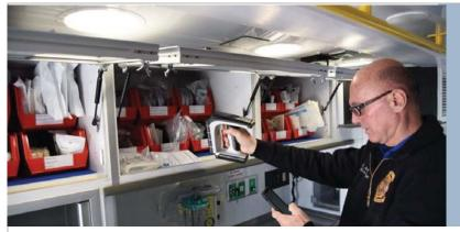
RFID readers and mounted gateway readers together produce a unique setup that provides the best tracking results. Each time an RFID tagged asset crosses through a reader entry point, its data is captured and time-stamped. Leveraging the cloud allows for quick updates to the data, and provides real-time locations of each asset.
