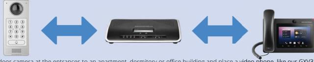
Put a door camera at the entrances to an apartment, dormitory or office building and place a video phone, like our GXV3275, in the apartments, dorm rooms or offices to allow visitors to be easily let in while also keeping the facility secure. The whole network is registered to and anchored by the UCM series IP PBX.
