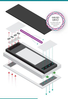
UV-C technology has been used as a disinfection method for decades. The UV-C wavelength of 253.7 nanometers has been proven to be effective at neutralizing dangerous microorganisms. The challenge with UV-C technology has always been the method of delivery. It can't be used in occupied spaces and is only effective on direct line of sight areas. Until now!
