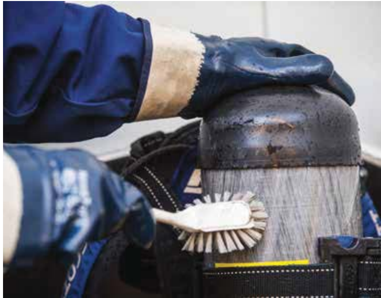
In the absence of a washer, manual washing is an alternative for decontaminating the breathing apparatus.
