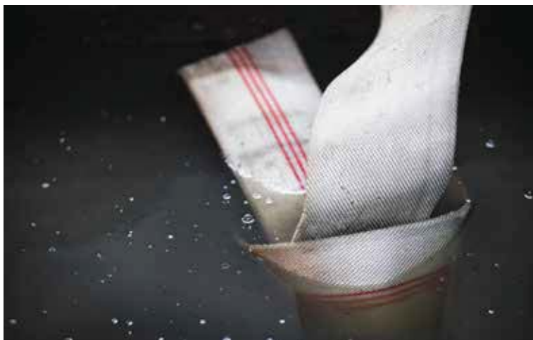
The coarse surface of the fire hose means that soot, ash and other waste from a fire are easily gathered.
