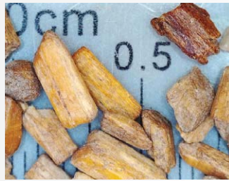
BrockFILL after 20,000 Lisport cycles.
