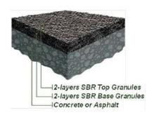
DynaFasTrack™ is a durable, resilient, textured, all weather system of permeable design consisting of four layers (2-layers base granules, 2-layers top granules) of recycled SBR black rubber granules bound with a latex spray.
