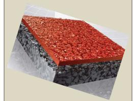
**DynaTrack-S2™:** A two layer, 13 mm, permeable spray coat track system. The base layer consists of black mat of SBR rubber granules bound in polyurethane. The surface layer is made up of polyurethane and colored EPDM granules applied by spray to provide a structural top-coat.
