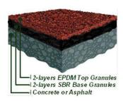
DvnaFasTrack-2C™ is a latex bound rubber track surface in which the top two layers of the system are colored EPDM rubber granules and the base are SBR lavers black rubber granules that are bound with latex. This produces а durable. resilient. textured. allweather. system permeable design.
