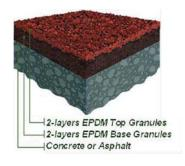
DynaFasTrack-FDC™ is a latex bound rubber track surface in which all layers consist of colored EPDM rubber granules that are bound with latex. This premium quality full depth color system produces a durable, resilient textured, all-weather running surface of permeable design.
