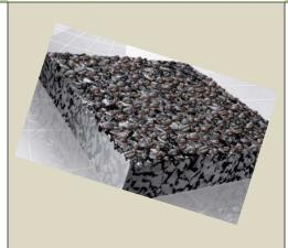
**DynaTrack-S1B™:** A single layer, 13 mm, permeable black mat track system consisting of SBR rubber granules bound in polyurethane.
