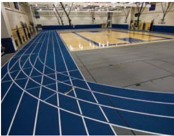
Prefabricated rubber sport surface made from synthetic & natural rubber compounds.
