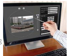
Canon's Remote Adjustment Function is a mechanical system that allows you to adjust camera position, zoom, and focus via your PC.
