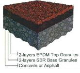
DynaFasTrack-2C<sup>™</sup> is a latex bound rubber track surface in which the top two layers of the system are colored EPDM rubber granules and the base layers are SBR black rubber granules that are bound with latex. This durable. produces а resilient. textured. allweather, system of permeable design.
