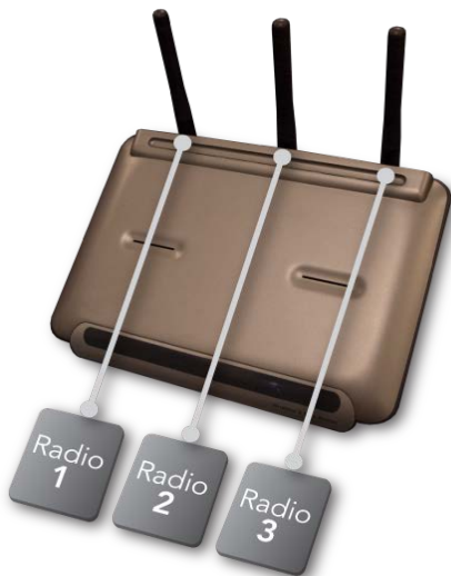
Fixed 1:1 relationship between Wi-Fi radios and antennas
