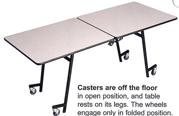
**Casters are off the floor** in open position, and table rests on its legs. The wheels engage only in folded position.
