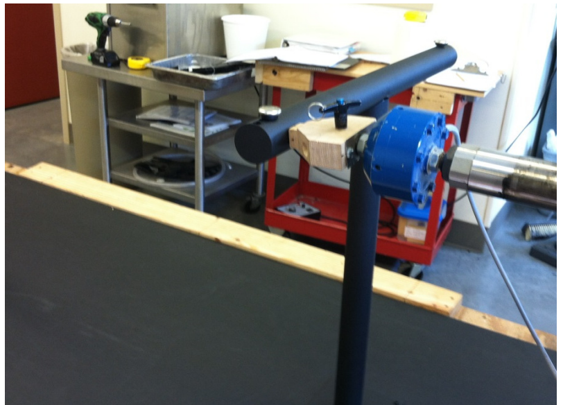
8: Rectangle Table Front Left Function & Proof Load
