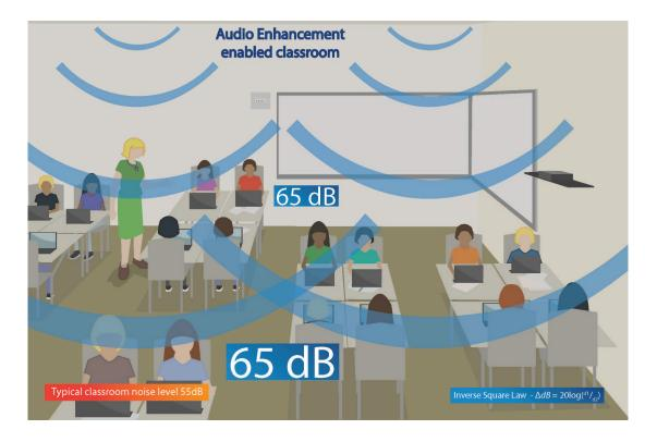
Sound technology is not about making the teacher's voice louder; it's about distributing that sound clearly and equally. At its core, the Inverse Square Law states that as the distance from a source of sound doubles, it is reduced to a quarter of its original intensity.
