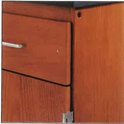
SQUARE EDGE OAK, 3MM OAK EDGE BAND, LUMBER CORE, PARTIAL OVERLAY, MORTISED HINGE
