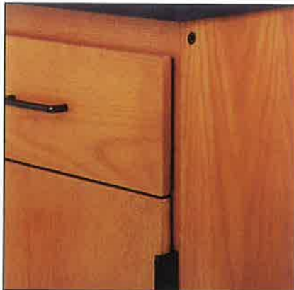
SQUARE EDGE OAK, 3MM OAK EDGE BAND, PARTICLE BOARD CORE, PARTIAL OVERLAY
