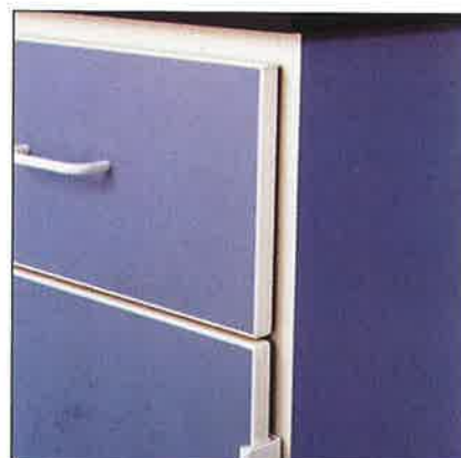
PLASTIC LAMINATE, 3MM TWILIGHT PVC EDGE BAND, PARTICLE BOARD CORE, PARTIAL OVERLAY
