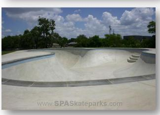
The transitional area of the College Station Skate Park consists of two unique bowls: a large, down-hill flow bowl and swimming pool replica. The flow bowl features a 10 ft deep end with a 14 ft extension, a bank wall, spine, and pool coping. The pool replica has an organic, free-flowing shape and features stairs, tile, and pool coping throughout.
