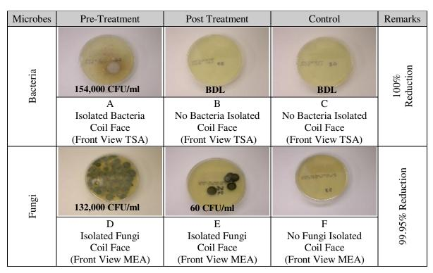
Figure 2. Effect of steam on microbial contaminants (A-F)
