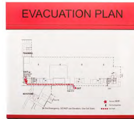
Regulatory and life-safety signs assist staff and visitors to egress safely during an emergency.
