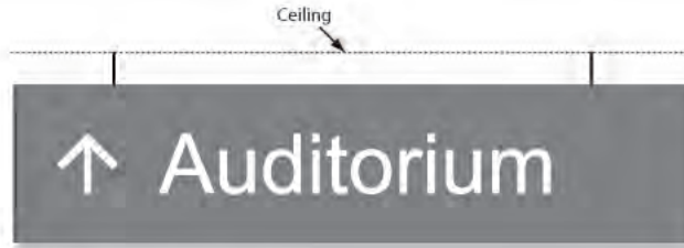
S.16 Wayfinding Ceiling Mount 8" x 34" Arc signs have edge rails on the top and bottom.
